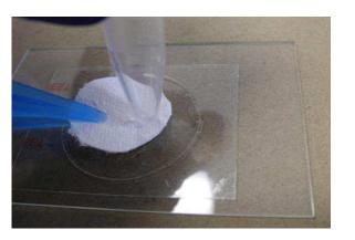
**Taming material being** applied to adhesive
