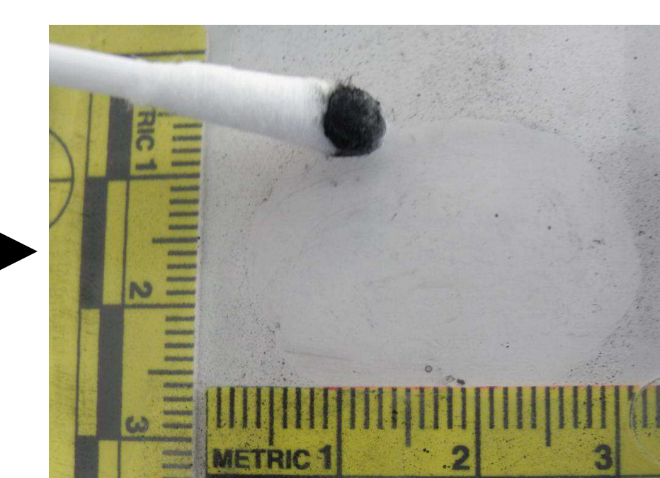
Collect leftover material using swab and OneTouch NDLB collection buffer.
